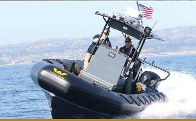
The multi-chamber tube is exceptionally strong and puncture resitant, providing maximum performance at sea and stability for boarding and equipment transfers.
